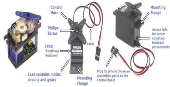
**Figure 3** The internal devices of a servomotor
